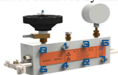
(Figure 5.1.5) Bolt tightening sequence
