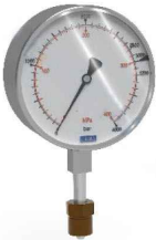
(Figure 2.1.1) Pressure gauge
