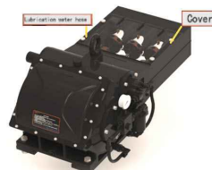
(Figure 3.2.3) Remove the lubricating water pipe
